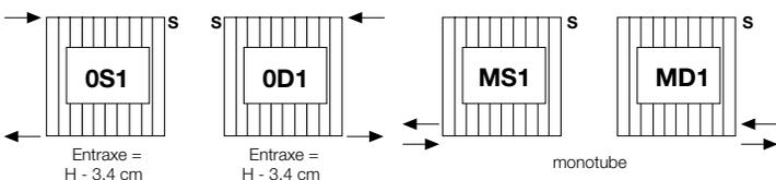
→ = Position des raccords S = Purgeur Air I = Entraxe raccords
